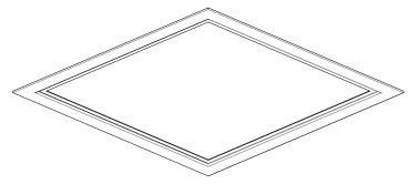
6. Lower LED light panel onto outer edges of frame, ensuring a secure fit.
