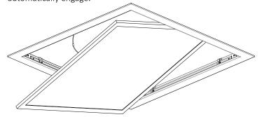
5. Angle LED light panel into frame and plug in power supply.
