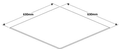
1. Neatly cut hole in gyprock ceiling.
