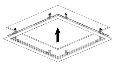
3. Carefully push frame up into hole - the spring clips will automatically engage.
