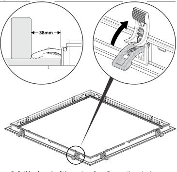
2. Pull back each of the spring clips. Ensure there is clearance around the hole in the gyprock for the clips to engage.
