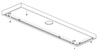
1. Fix frame to ceiling in desired location using appropriate fixings suitable for the ceiling material.
