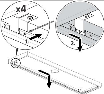
2. Undo grubs screws that hold frame to the surface mount hangers and slide frame across and down to remove.
