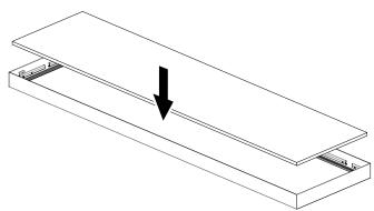
3. Assemble LED light panel into the frame.
