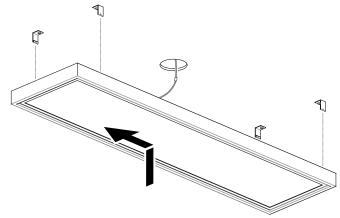
4. Lift frame up towards the ceiling, plug in power supply then locate frame on surface mount hangers and slide across
