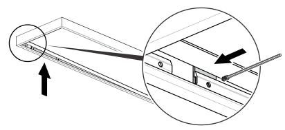
5. Tilt LED light panel and ensure frame is aligned with the surface mount hangers, then secure frame to the hangers with grub screws.
